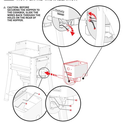
⚠ BEFORE FULLY TIGHTENING THE SCREWS, PULL ANY OF THE EXTRA WIRES INTO THE HOPPER AREA. DO NOT CRUSH OR KINK ANY OF THE WIRES.
