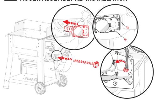
**⚠ CAUTION: CAREFULLY PLUG IN THE** CONNECTOR(S), DO NOT DAMAGE THE PLUG WHEN RECONNECTING IT TO THE GRILL.
